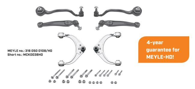
One control arm to replace its three OE equivalents. Easy wheel camber correction thanks to clear part marking:
