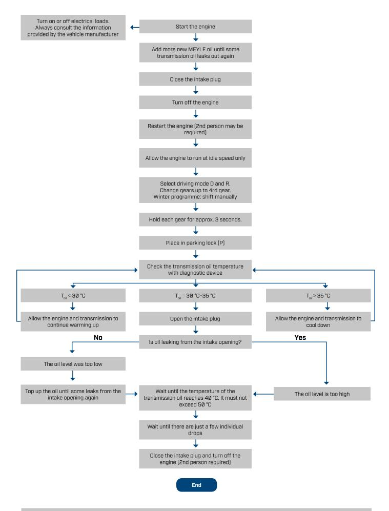
NB: Depending on the type of transmission, it may have a bypass valve which opens or closes the oil circuit to the oil cooler, which is why the drive should be sufficient to ensure the transmission oil temperature reaches at least 75 °C.
