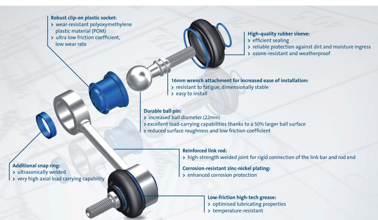
Our engineers are passionate about improving our MEYLE-HD stabilizer links constantly seeking new ways of refining all components. To make installation and removal procedures easier for our customers, more and more MEYLE-HD stabilizer links are designed with a wrench attachment at the ball pin. A distinguishing advantage, in particular over those original designswhich lack this value-adding feature.
